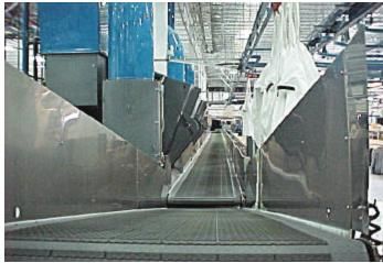
After a washer or a dryer has completed its cycle, the machine will look to see if there is a means to unload. The machine will send an invitation to be unloaded. If the conveyors "Belt Empty" input is on, the conveyor will send an invitation to be loaded. This will start the unload sequence.
